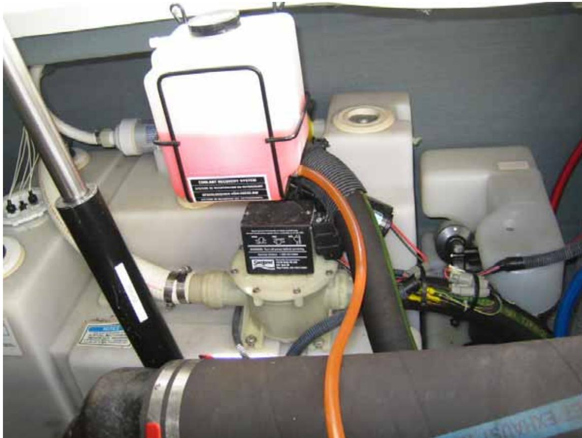
Photo 14. Vacuflush system and water tank to port in engine room.
