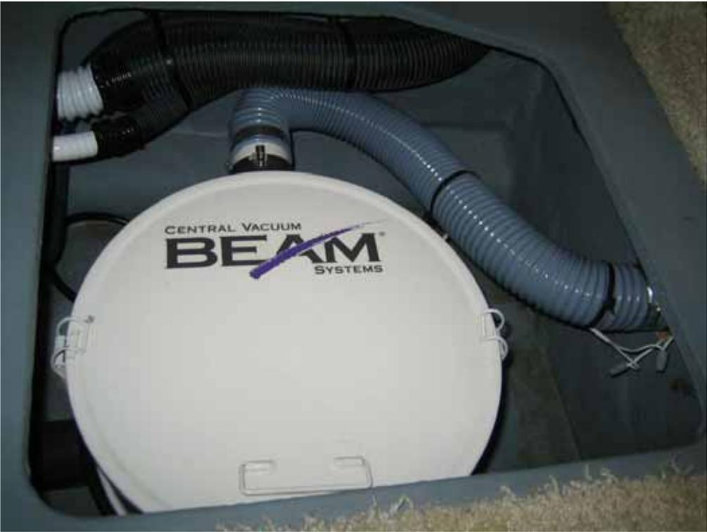
Photo 20. Central vacuum located under aft cabin seat.
