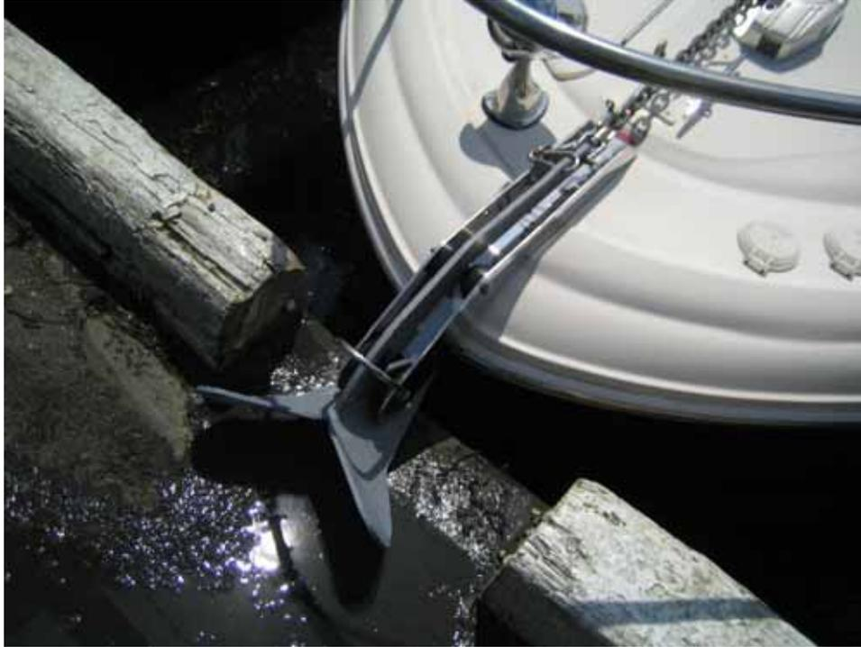
Photo 10. Delta style plow anchor and bracket.
